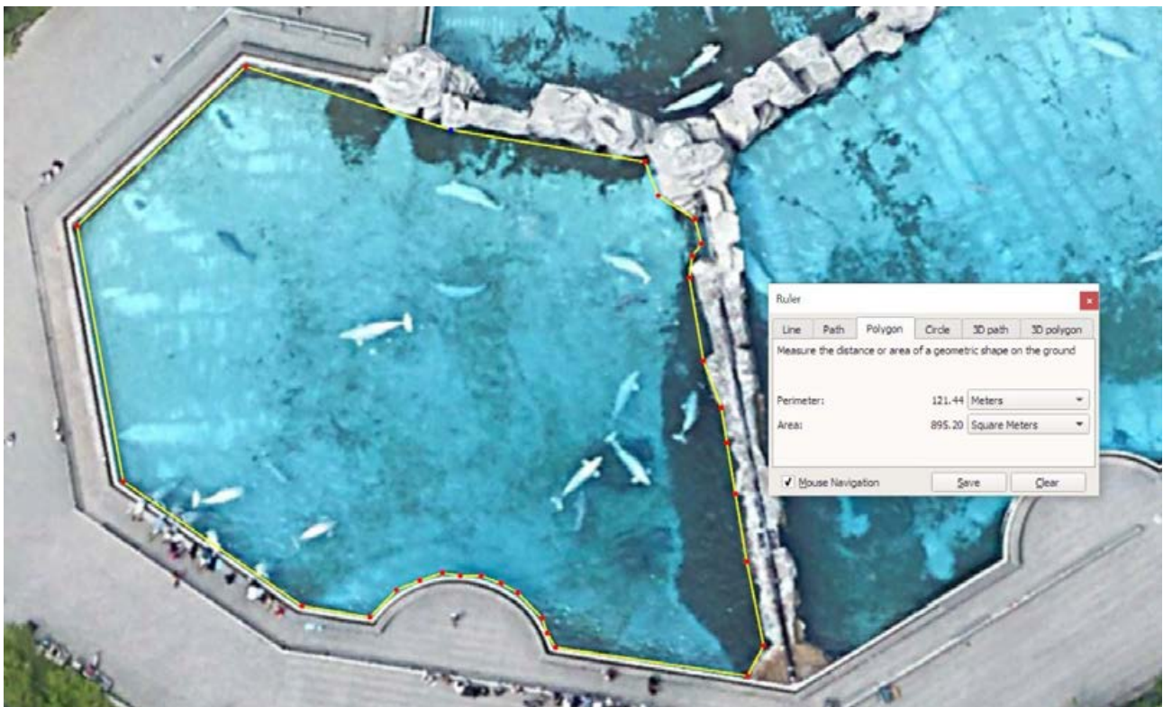
Figure Dc. At Arctic Cove, the West tank has a minimum perimeter of 121.44 m and a minimum surface area of 895.20 m 2 .
