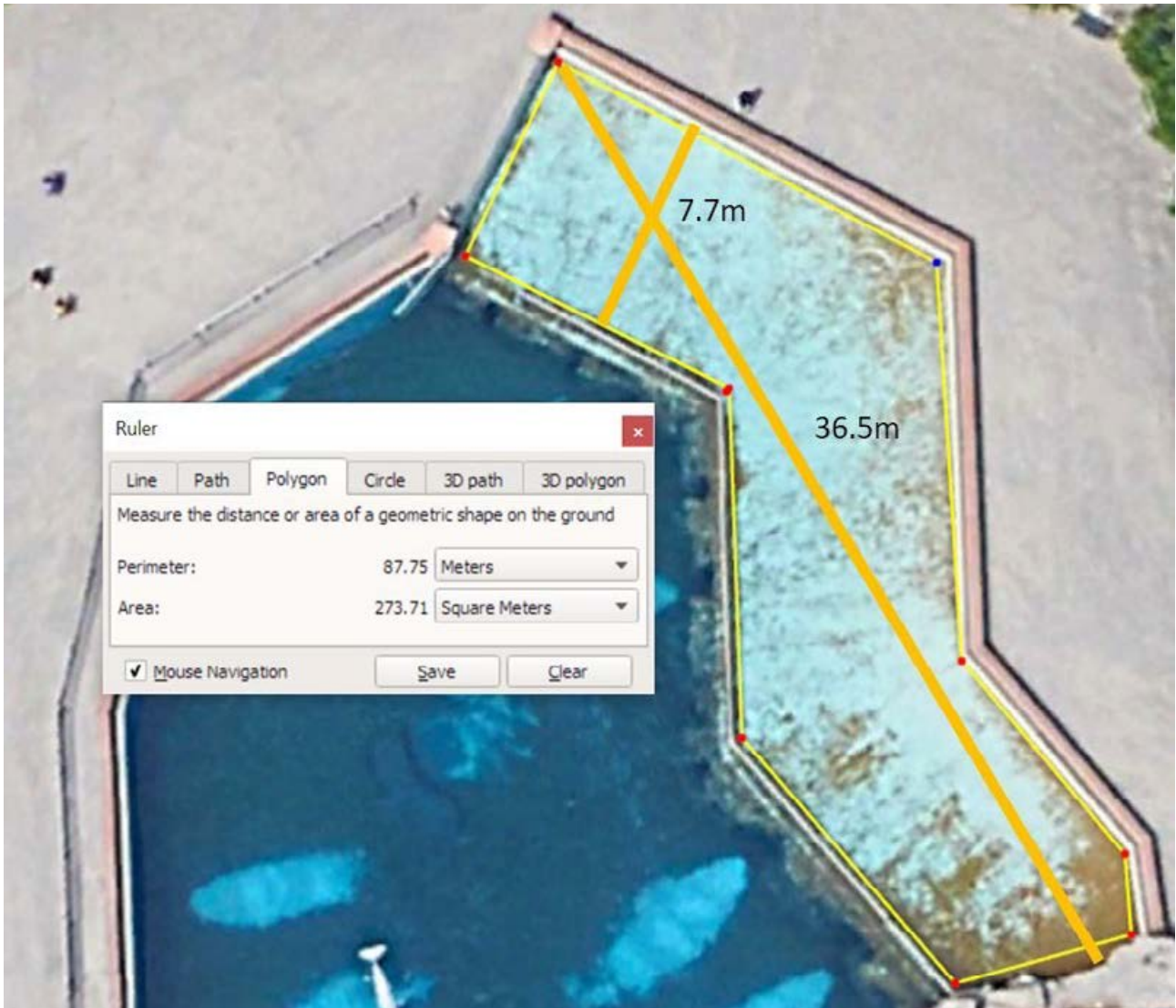
Figure Ce. At Friendship Cove, the North medical tank has a minimum perimeter of 87.75 m and a minimum surface area of 273.71 m 2 . The maximum length is 36.5 m and the maximum width is 7.7 m. No cetaceans can be seen in this tank. Measurements from Google Earth.
